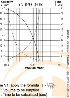
To calculate the emptying time of a volume V1, apply the formula  $1 = \frac{1 \times V_1}{100}$ V1 : Volume to be emptied
